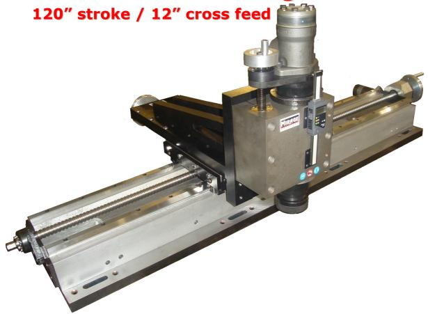
A 3 axis milling machine that is built for rigidity and accuracy suitable for all all general purpose in situ milling. Used on heat exchangers, pump and motor pads, steel mill stands, ship building, turbine split lines and many more applications.
